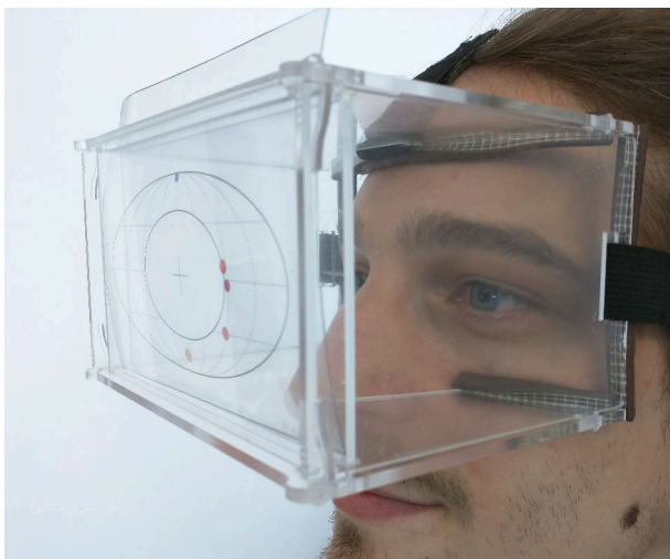
Figure 4: Person wearing our lo-fi AR prototyping tool. Best seen in color.
