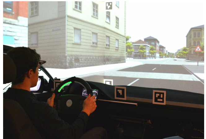
Figure 1: Participant driving in the simulator using ambient light navigation on the steering wheel.
